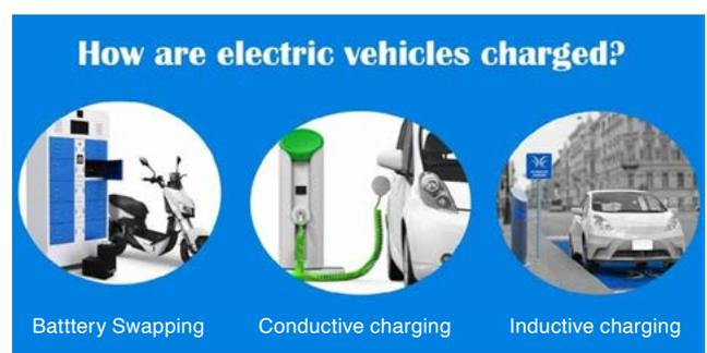
Figure 8: Basic charging solutions: battery-swapping, conductive and inductive charging.
