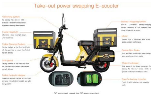
**Figure 33:** Two-wheeler with battery-swapping.
