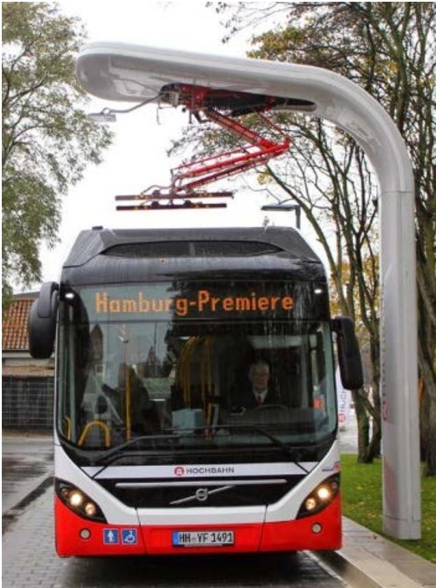
**Figure 32:** Bus undergoing conductive charging. (Electric Vehicle News, 1014).
