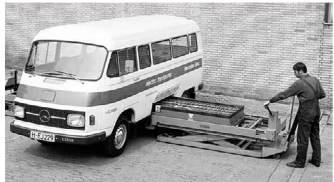
**Figure 25:** Mercedes-Benz battery-swapping solution in the 1970s (Sandru, 2009).
