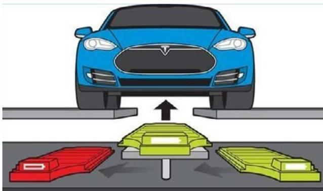
**Figure 29:** Operation of Tesla battery-swapping. (Luxury Perspective, 2014).
