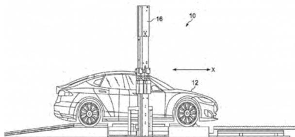
**Figure 28:** Tesla battery-swapping solution. (Owano, 2017).
